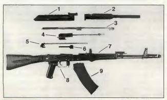
Main parts and assemblies of the AL-7: 1 — top cover with rear sight, 2 — gas tube with steel cover, 3 — upper rail with gas piston, synchronizing sprocket and return spring, 4 — bolt carrier with gas piston, 5 — return mechanism of bolt carrier, 6 — bolt, 7 — barrel with receiver, stock and hand-guard, 8 — trigger and trigger mechanism, 9 — magazine.
